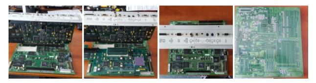
Ultrasound machine uses 50pin SCSI disk connected to on-board SCSI2 controller. Disk is split into 4 FFS partitions and uses original Amiga OS 3.1. But Startup-Sequence is re-written to launch the application from the beginning, so Workbench is not loaded at all. OS contains special 68040 and 68060 libraries, special DSP.device drivers and it also Turboprint application installed (via parallel device). Other stuff is then stock OS3.1.
