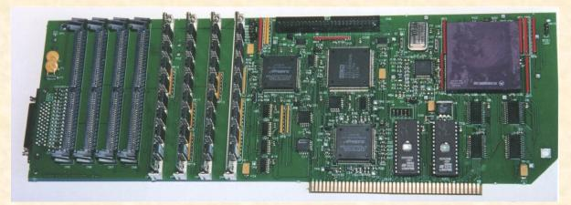
When it works, it is very fast, and can easily be overclocked. Its SCSI controller has some limitations (like not being able to automount other filesystems than FFS), but it is also very fast (one of the fastest I have experimented on the various 68060 Amiga configurations I own) and bug free.
